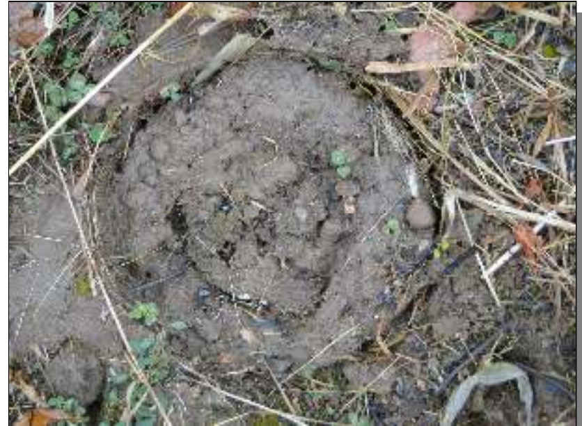
Photo 28: A double ring infiltrometer confirmed on 11-11-19 that the substrate on Work Pad #3 is much less pervious than natural hilltop soil.
